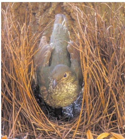
Figure 1 Robotic female satin bowerbird. Robots were capable of three movements, controlled by servo motors: crouching (simultaneous lowering and forward-tilting of the body), looking around during courtship (lateral head movement), and wing-fluffing upon reaching the mating position (lateral wing movement). Robots were enclosed in female satin-bowerbird skins, placed in the bower of the male under test (where females are typically courted 9 ) at our field site in Australia, and controlled remotely. The responses of 20 males were tested with robots that crouched from the upright position to the mating position (pictured) at four different rates: fast (3 min total, 1.67 position changes per min), moderate (6 min, 0.83 changes per min), slow (9 min, 0.55 changes per min), and no crouching (0 changes per min), with order randomized between males.
