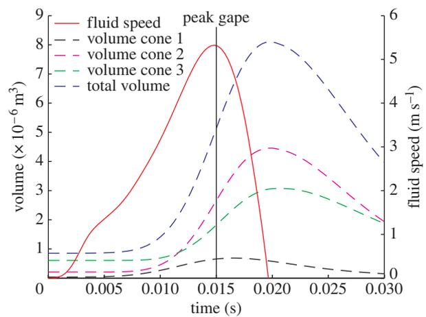
Figure 6. Buccal cavity volume change and fluid velocity at the mouth opening through a sample strike using a three-cone geometry. For this simulation,  $\alpha = 7$ , anterior cone length was 2 mm, onset delay for section 2 was 15% and onset delay for section 3 was 25% of total strike time. Peak velocity occurs just before peak gape and its magnitude is greatly reduced relative to figures 3 and 4.
