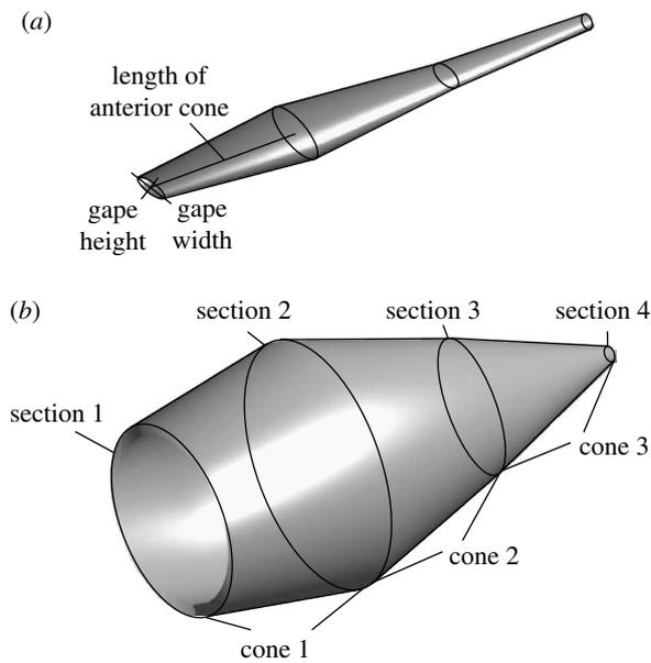
Figure 1. Buccal cavity geometry consisting of three interconnected, truncated, elliptical cones in (a) unexpanded and (b) fully expanded configurations. In this example, the length of the buccal cavity is roughly equally distributed between the three cones. In the computational model, the buccal cavity length can be distributed in any way between the three cones.
